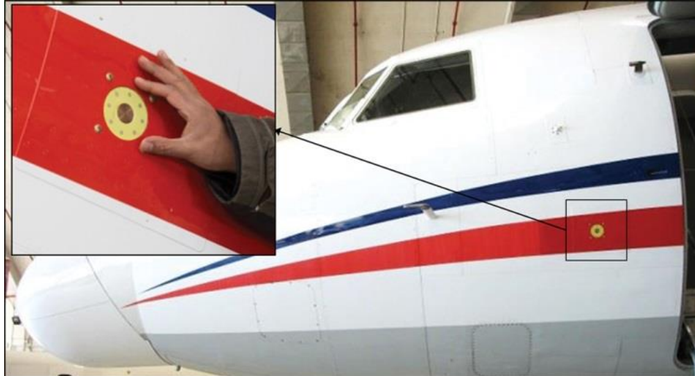
Figure 10: PDP installed on NRC Convair 580 Flight Test aircraft
