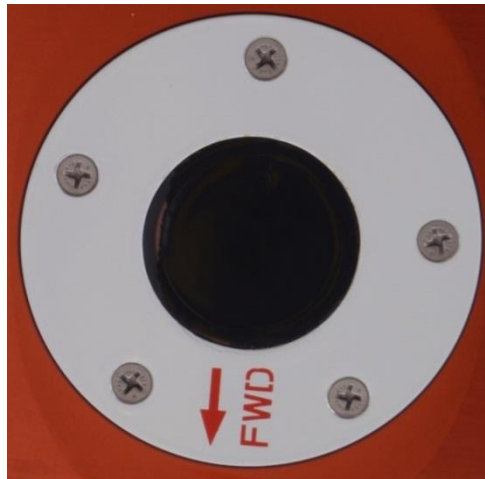
Figure 14: PDP with initial paint erosion due to particle impact
