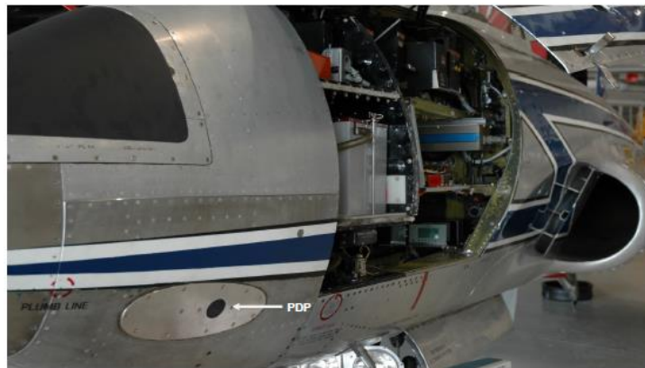
Figure 9: PDP probe installed on NRC CT-133 Aircraft
