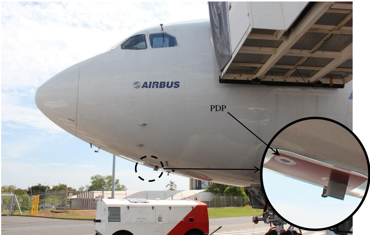
Figure 13: PDP installed on A340 flight test aircraft with inset zoomed in to show details
